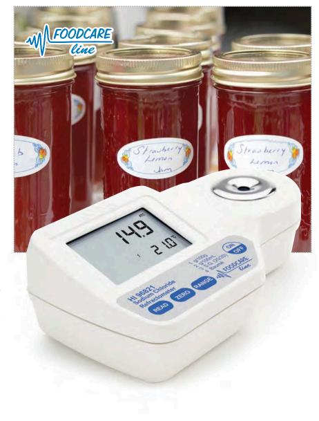
HANNA offers the HI 96821 digital sodium chloride refractometer to meet the requirements of the food industry. This optical instrument employs the measurement of the refractive index to determine sodium chloride concentration in aqueous solutions used in food preparation. It is not intended for sea water salinity measurements.
